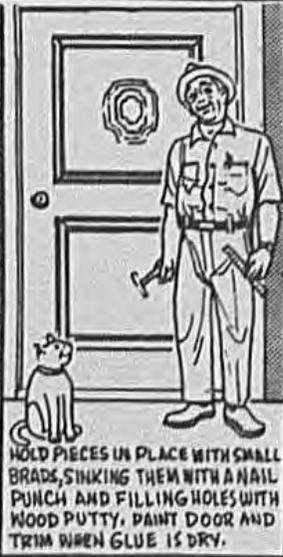
HOLD PIECES IN PLACE WITH SMALL BRADS, SINKING THEM WITH A NAIL PUNCH AND FILLING HOLES WITH WOOD PUTTY. PAINT DOOR AND TRIM WHEN GLUE IS DRY.
