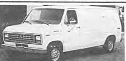
4.9 FUEL INJECTED 6 CYL. ENGINE AUTOMATIC TRANSMISSION DRIVER & PASSENGER BUCKET SEATS FIXED REAR DOOR GLASS 6100 LBS. GVWR PACKAGE ENGINE COVER CONSOLE ARGENT REAR STEP BUMPER
